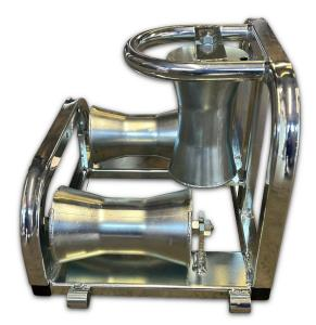
Heavy duty triple corner cable roller for use in most cable laying applications and for cables up to 130mm. These can be used singularly or linked together using link pins to form a full bend. All of the bend roller range have the same link points to facilitate various bend/roller configurations.
